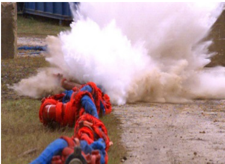
Destructive testing conducted with a designed failure at 22,500 psi on up to 4" iron utilizing SPM® FSR
